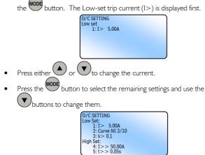
Actual LCD presentation when adjustable parameters are displayed. Screen example above also shows the default settings for OVERCURRENT
