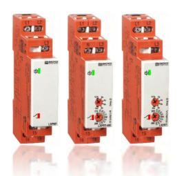
Not all applications require a product that offers all the features on the LXPRC/S. Therefore, in the LX range are models that monitor for just phase loss, phase reversal and under voltage or just simply, phase loss/reversal. In some instances, the requirement of the specifier may be that a product with only certain features be used in an application in order to keep things simple.
