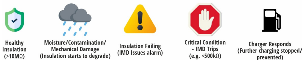
Figure 2 – Example of the progression from healthy insulation through degradation to a critical insulation condition.
